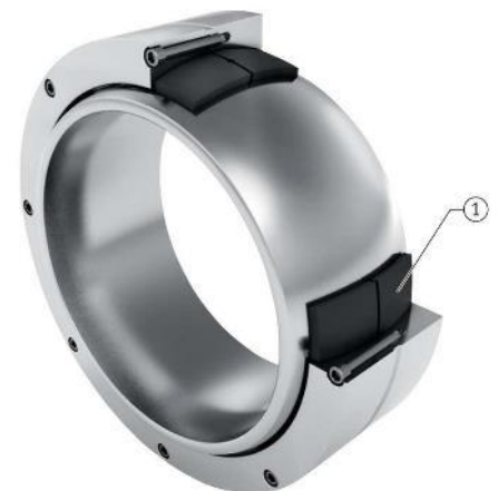
ELGES large spherical plain bearings with a sliding layer (1) made of glass-fiber reinforced plastic (GRP) and PTFE (GE..-DF series bearings)
