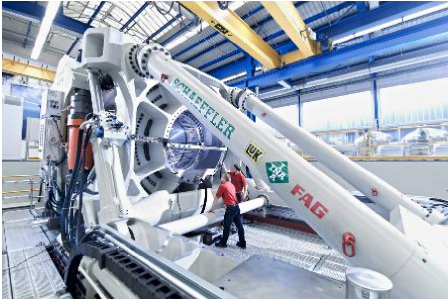
Fig. 6: Since 2011 Astraios has been delivering valuable findings that are used for developing new bearing solutions and optimizing simulation and calculation models thanks to its near-real power and torque simulation.
