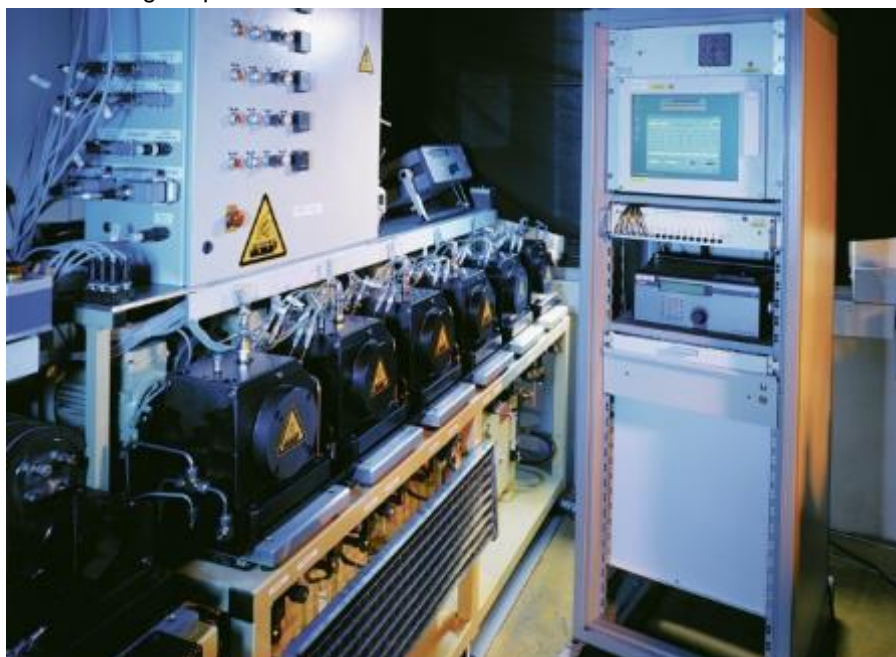
Fig. 3: Radial bearings in endurance testing – rating life test stand in the Schaeffler research and development center in Herzogenaurach.
