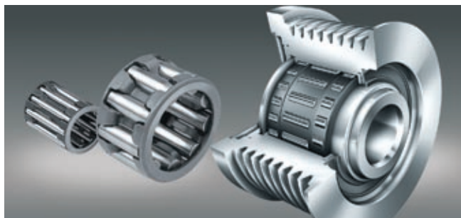
Increase engine operating life: Crank pin cage for extreme accelerations and pulley for decoupling the generator from the rotational irregularities of the crankshaft
